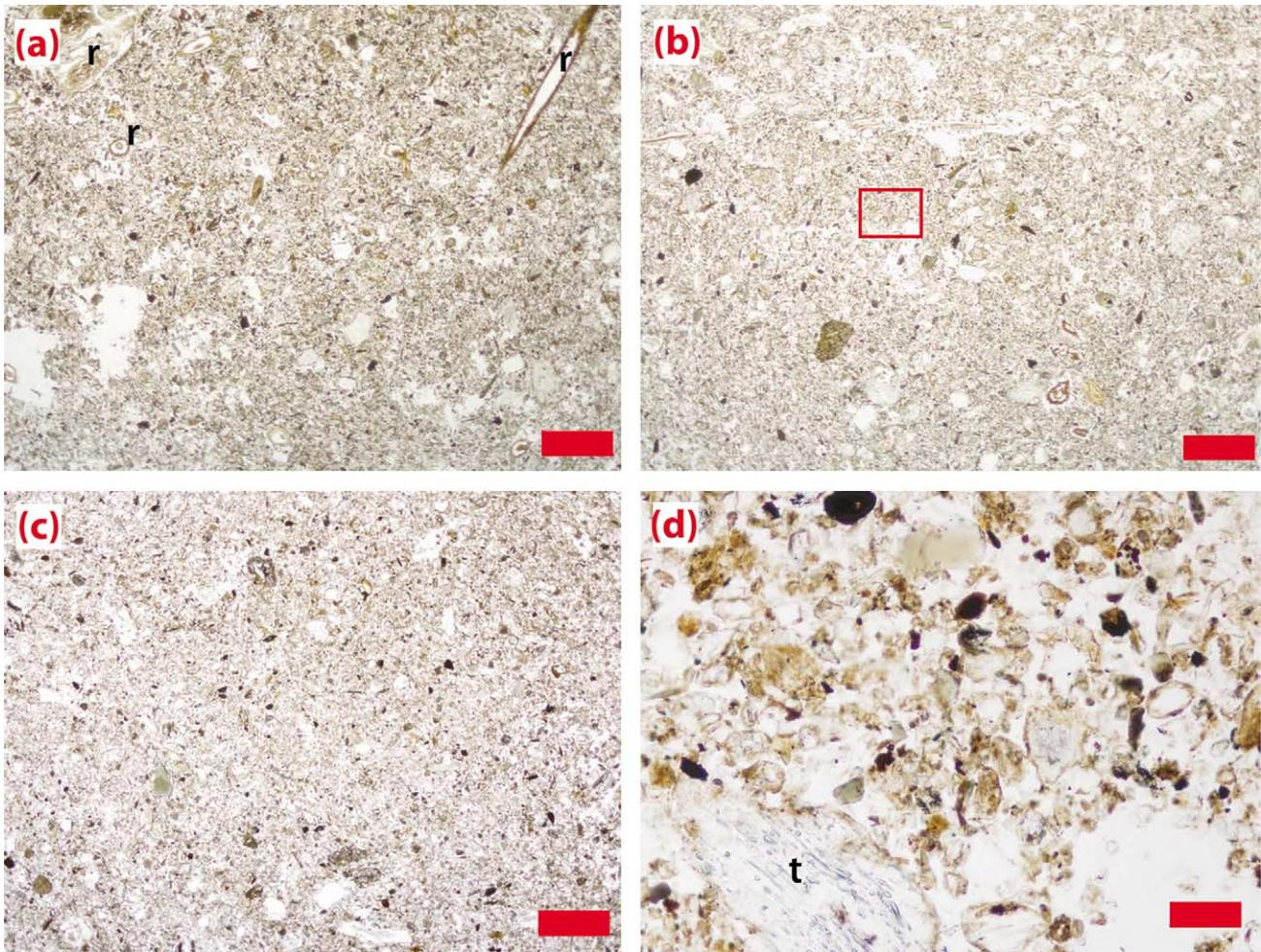
**Fig. 5.** Micrographs (plane light) of thin sections from Kluane pedon: (a) Ah horizon, ~1.0–1.5 cm depth; (b) Ah horizon, ~5.0–5.5 cm depth, with rectangle outlining detail of coated sand, silt, and tephra particles shown in (d); (c) Ck horizon, ~43.5–44.0 cm depth. Abbreviations: r, root; t, tephra. Scale bars: 1.0 mm (a, b, c), 0.1 mm (d).
