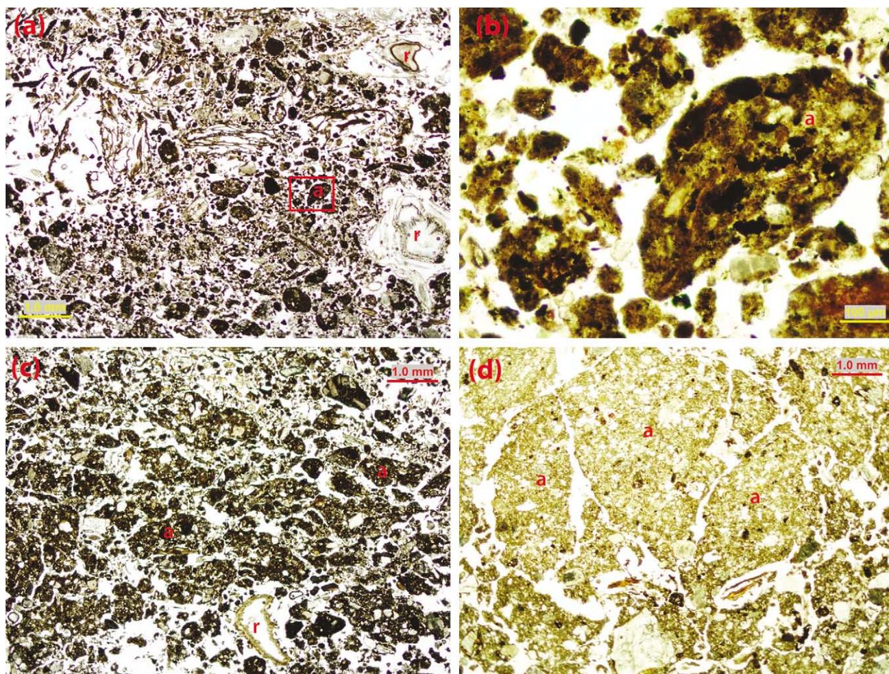
**Fig. 3.** Micrographs (plane light) of thin sections from Stikine pedon: (a) Ah1 horizon, ~0.5–1.0 cm depth, with rectangle outlining detail of crumb microstructure shown in (b); (c) Ah1 horizon, with aggregates ~1–2 mm long; (d) Ah2 horizon, with subangular blocky microstructure. Abbreviations: a, aggregate; r, root. Scale bars: 1 mm (a, c, d), 0.1 mm (b).
